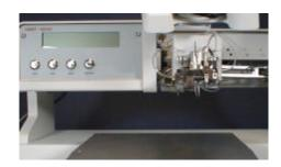
**UNLIMITED DEEP REACH** access to remote bond targets on large packages with WEST-BOND'S new throatless chassis and micromanipulator designs. All machine components, circuitry, and enclosures are arrayed above the horizontal bond plane, eliminating any restrictions to package size or shape. Manual "E" Series models are available for all microwave, semiconductor, R.F., and hybrid production, and are ideal for repair station or laboratory use.
